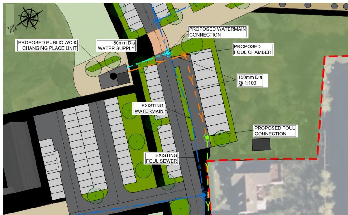
Figure 3-1 Proposed water supply and foul drainage connections
